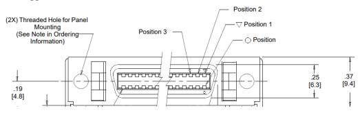
Figure 5 26-pin 3M Mini-D Ribbon connector
