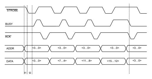
Figure 2 Sending list word over FCP in '8-bit Mode'
