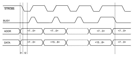
Figure 4 Programming of frequency list over FCP in '16-bit Mode'
