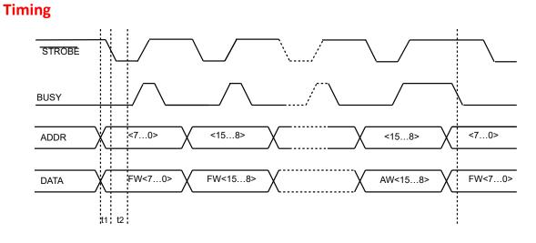
Figure 3 Programming of FW with FCP in '16-bit Mode'
