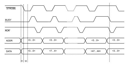
Figure 1 Programming of FW over FCP in '8-bit Mode'
